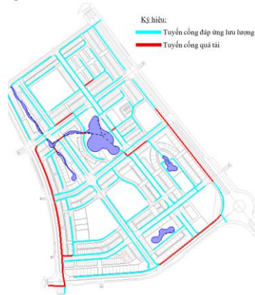
Figure 7. Simulation Results of the Drainage Network after the Application of the SPC Model
