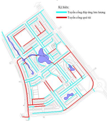
Figure 6. Simulation Results of the Drainage Network before the Application of the SPC Model
