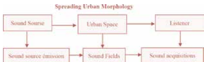
Figure 2: The role of the acoustic channel between the sound source and the sound acquisition
