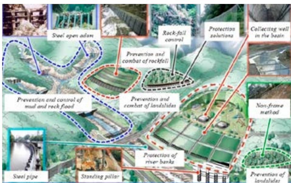
Figure 6. Planning diagram of solutions to prevent rock falls, landslides, and flash floods in Japan [4]
